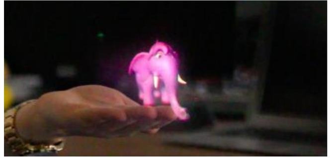
Fig. 3. Augmented Reality Holographic Elephant Image. Photographed directly through the eye-piece with DSLR camera. Image is constructed by overlaying RGB holographic elephants in the replay field to create single full-colour elephant.
